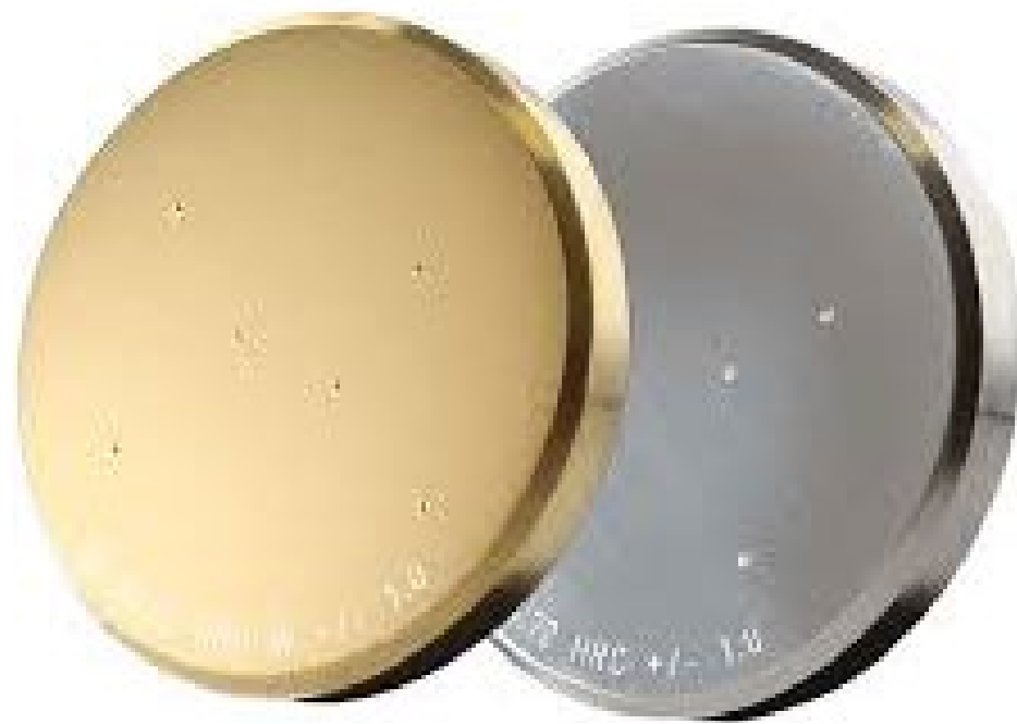
Figure 1. Example brass and steel hardness test blocks.
